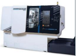
**THE MANURHIN K'MX 1032** is delivered in two versions –one for bars Ø 32 and one for bars Ø 36 mm (bar preparation is needed). The highlight of the K'MX 1032 is the productivity. Up to 25 tools (including up to 17 powered tools) can be working simultaneously with 10 independent axes. Tool changes are quick and easy with the compatible tool holder cartridge system. The large door opening provides easy access to tools for operator.
