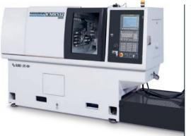
**THE MANURHIN K'MX 532 TREND** is designed for productive machining of parts for bars with a maximum diameter of 32 mm. With a spindle bore diameter of 37 mm, no modification of the end of the bar for bar feeder collet is needed. The machine comes standard with two electro spindles, each with a maximum speed of 10,000 rpm and with a rotary guide bush, synchronized by pulleys and belts from the main spindle. Five linear axes (X1, Y1, Y2, Z1, Z2) two rotary axes (C1, C2).
