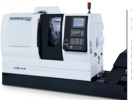
**THE MANURHIN K'MX 816 CLEVER** is designed for the productive machining of parts for bars of a maximum diameter of either 16mm or 20mm. The machine comes standard with two electro spindles and a rotary guide bush that is synchronized by pulleys and belts from the main spindle. Eight linear CNC axes (X1, X2, Y1, Y2, Y3, Z1, Z2, Z3) and two rotary axes (C1, C2) enable the machine to produce parts ranging in complexity. The construction solution enables the use of 4 tools at the same time.
