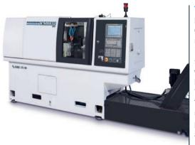
**THE MANURHIN K'MX 632 DUO** is designed for productive machining of parts for bars with a maximum diameter of 32 mm. With a spindle bore diameter of 37 mm, no modification of the end of the bar for bar feeder collet is needed. The machine comes standard with two electro spindles, each with a maximum speed of 10,000 rpm and with a rotary guide bush synchronized by pulleys and belts from the main spindle. Six linear CNC axes (X1, X2, Y1, Y2, Z1, Z2) and two rotary axes (C1, C2).
