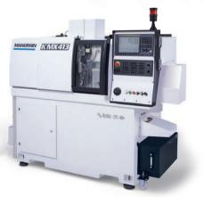
**THE MANURHIN K'MX 413** is dedicated to run small parts from  $\emptyset$  3 (2)–16 mm (over  $\emptyset$  13 mm, preparation of bars is necessary in standard, as an option it can be used with full  $\emptyset$  16mm bars without preparation). Counter spindle, powered tools are included in the basicmachine as well as the barloader.
