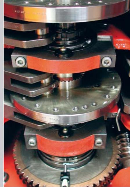
■ Drives of longitudinal slides – all four branches of the drives of slides are protected with independent overload release clutches
