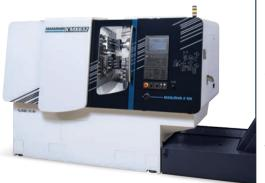
**THE MANURHIN K'MX 632** is designed for productive machining of parts for bars with a maximum diameter of 32 mm. With a spindle bore diameter of 37 mm, no modification of the end of the bar for bar feeder collet is needed. The machine comes standard with two electrospindles, each with a maximum speed of 10,000 rpm and with a rotary guide bush, synchronized by pulleys and belts from the main spindle. Six linear axes (X1, X2, Y1, Y2, Z1, Z2), two rotary axes (C1, C2).
