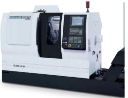
THE MANURHIN K'MX 816 CLEVER is designed for the productive machining of parts for bars of a maximum diameter of either 16 mm or 20 mm. The machine comes standard with two electrospindles and a rotary guide bush that is synchronized by pulleys and belts from the main spindle. Eight linear CNC axes (X1, X2, Y1, Y2, Y3, Z1, Z2, Z3) and two rotary axes (C1, C2) enable the machine to produce parts ranging in complexity. The construction solution enables the use of 4 tools at the same time.
