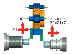
SolidCAM supports three different superimposition modes. A pair of axes can be superimposed one to another, where the slave one follows the master one. For applicable Mill-Turn machines, SolidCAM will automatically detect this mode.
