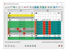
The Channel Synchronization's clash engine displays any issue with logical comments. The intelligent system holds the logic and checks the possibilities of the synchronization taking into account the complete machine kinematics.
