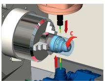
Reduce machining time by sharing axes and drive units. Synchronize your milling/turning operations, on different turrets, on the same table device, under specific conditions.
